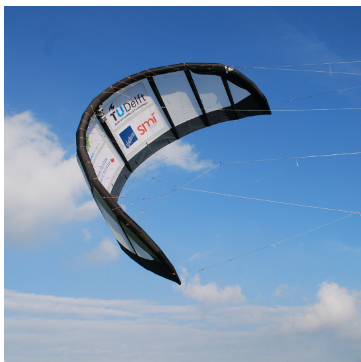
Figure 1: The KitePower is an example of a wind energy system concept that consists of a thin membrane structure [2].
