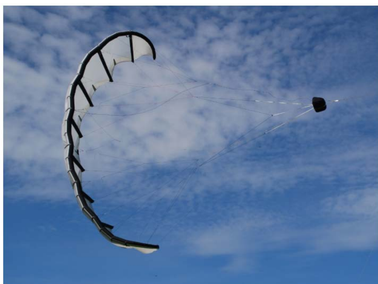
Figure 1: The TUD-25mV3 LEI kite in flight (Photo: R. Schmehl).
